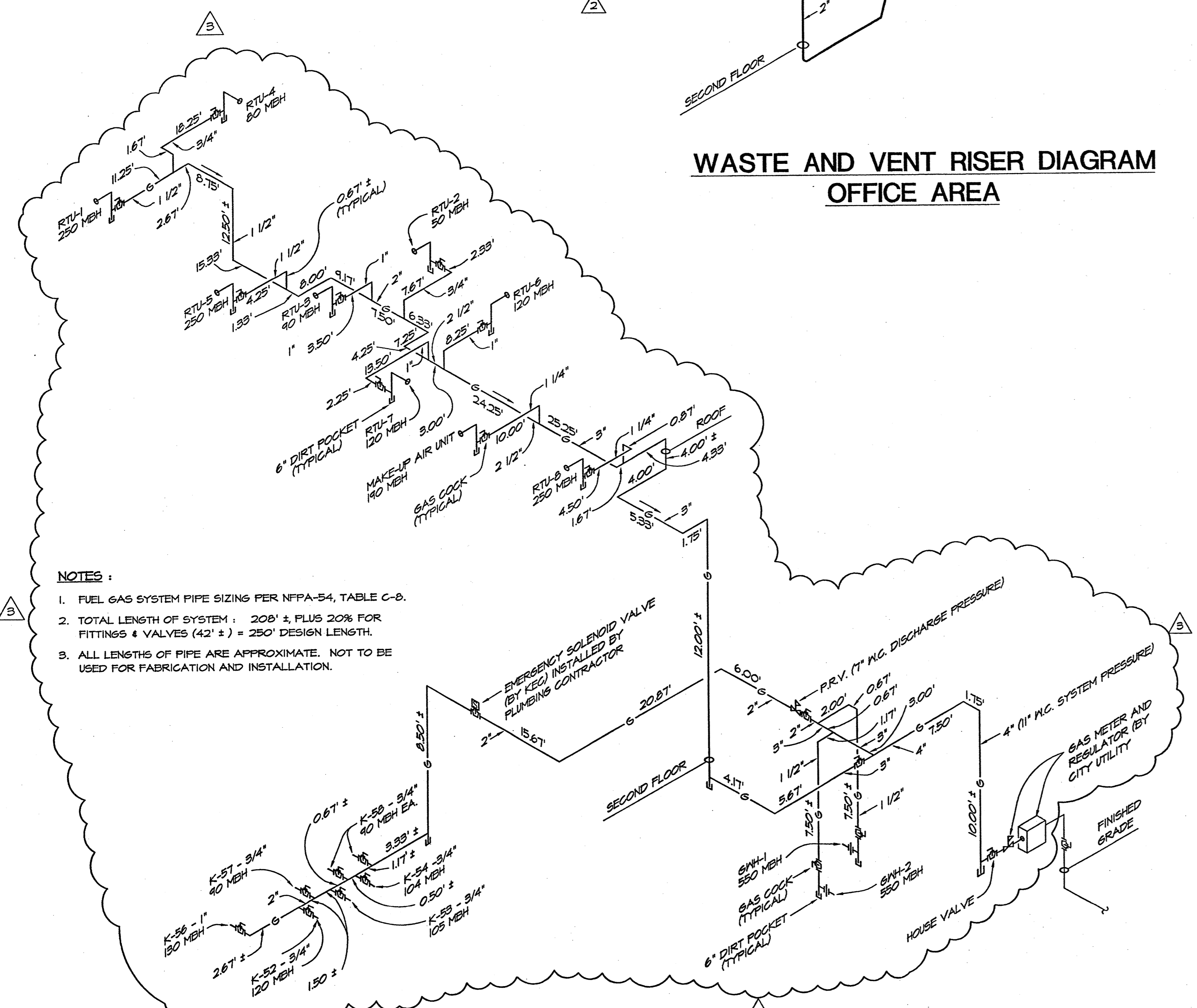
GAS RISER DIAGRAM
